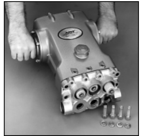
Rotate Crankshaft to position plungers
