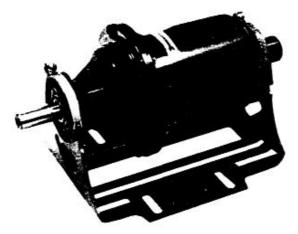
**Storage.** Always drain pump for extended storage periods by removing suction and discharge lines, loosening resilient mount clamps and turning discharge port to drain position.
