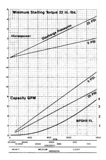
NOTE:For fluids with viscosity over 200 CP (1000 SSU), pump capacity is reduced by 20%.
