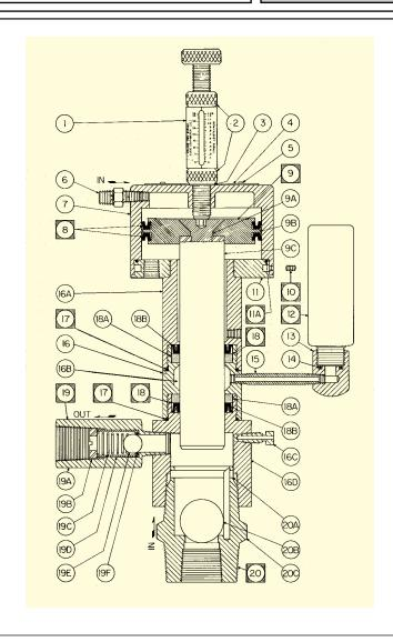
**LUBRICATION:** All pumps are supplied with SF96-100 plunger seal lubricant. Use G321M1 U-cup silicone grease when rebuilding the pump. This is contained in a complete pump repair kit.
